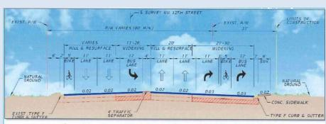
Figure 6-1 Proposed Typical Section from Dolphin Station Road to HEFT
