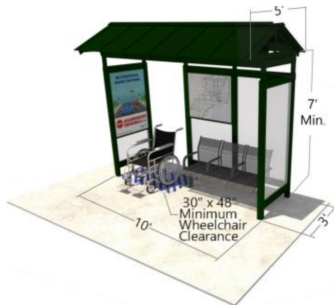
Figure 3- 7: General Minimum Requirements for Shelters
