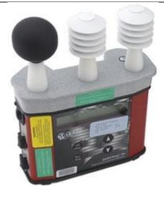
Figure 3: Waterless wet-bulb meter
