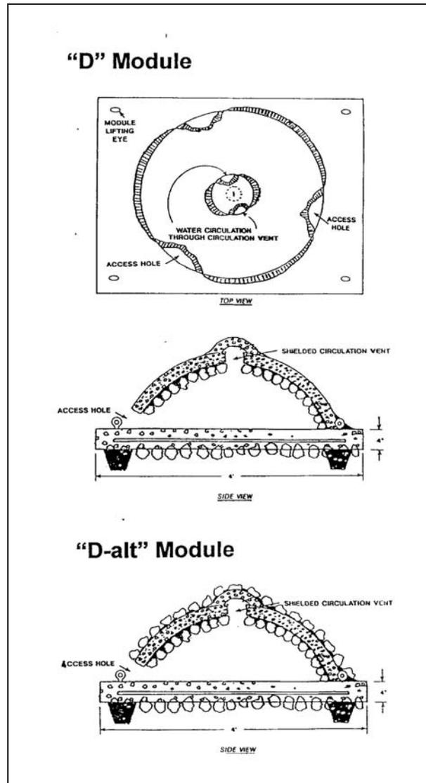
**Figure 5:** Dome Module (D) diagram (Selby and Associates, Sunny Isles Artificial Reef Monitoring Program: 8<sup>th</sup> Quarterly Report, 1994). The "D" module, or the smooth dome, lacks the cobbled, exterior surface. The "D-alt" module, or the rough dome, has the cobbled, exterior surface.
