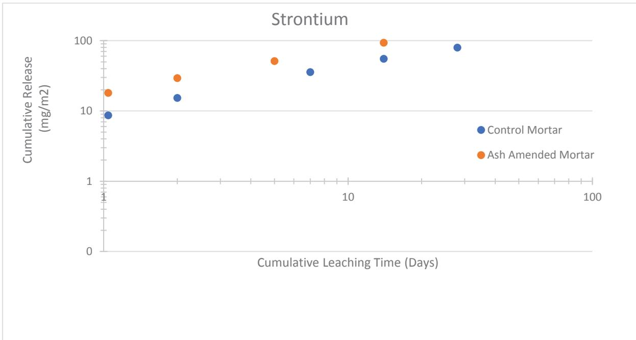
**Figure B-12. Cumulative mass release for strontium, EPA Method 1315, for control and ash-amended mortar specimens**
