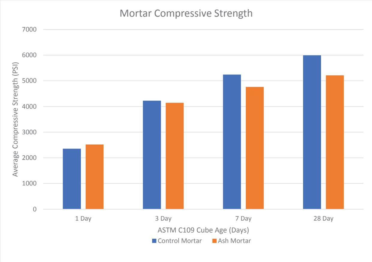
**Figure 4.4. Evolution of mortar compressive strength over time**
