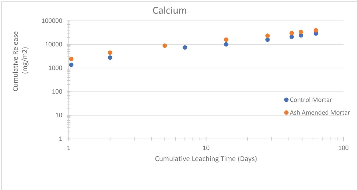
**Figure B-3. Cumulative mass release for calcium, EPA Method 1315, for control and ash-amended mortar specimens**
