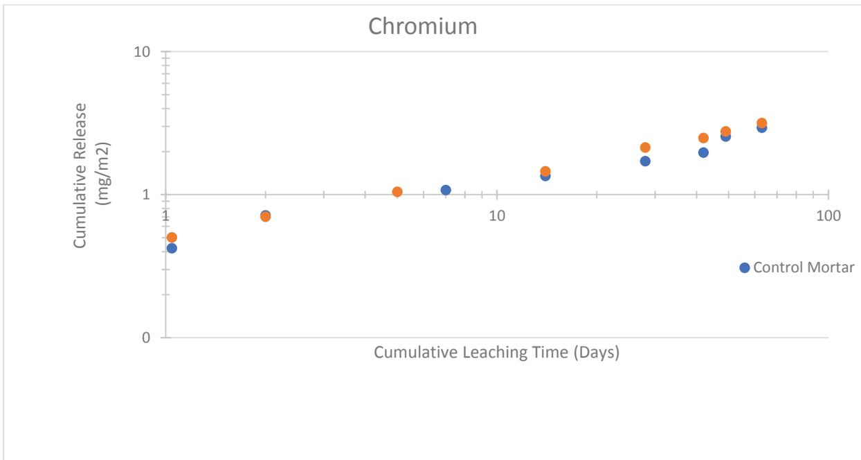
**Figure B-4. Cumulative mass release for chromium, EPA Method 1315, for control and ash-amended mortar specimens**
