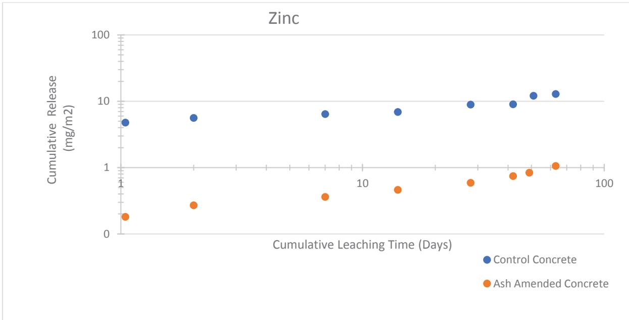
**Figure C-14. Cumulative mass release for zinc, EPA Method 1315, for control and ash-amended concrete specimens**
