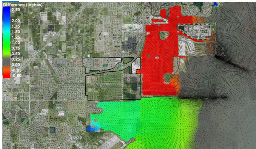
Figure 13 Differences in Surge Elevations for with and without project for Storm #33 (positive number is an increase in elevation due to project)
