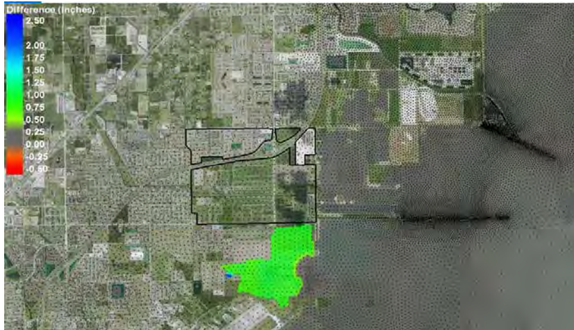
Figure 15 Differences in Surge Elevations for with and without project for Storm #248 (positive number is an increase in elevation due to project)
