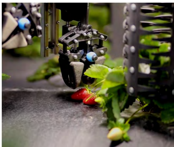
Figure 25. HCR mechanism for moving leaf foliage (right) and an end effector of a picking robot (left).
