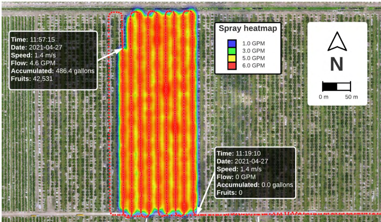
Figure 10. Example of a spraying heatmap for a 5.44-hectare citrus orchard.
