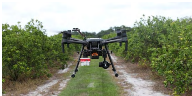
Photo of unmanned aerial vehicle equipped with multispectral camera for assessing crop conditions, pests and diseases. (Source: Ioannis Ampitzidis, University of Florida).
