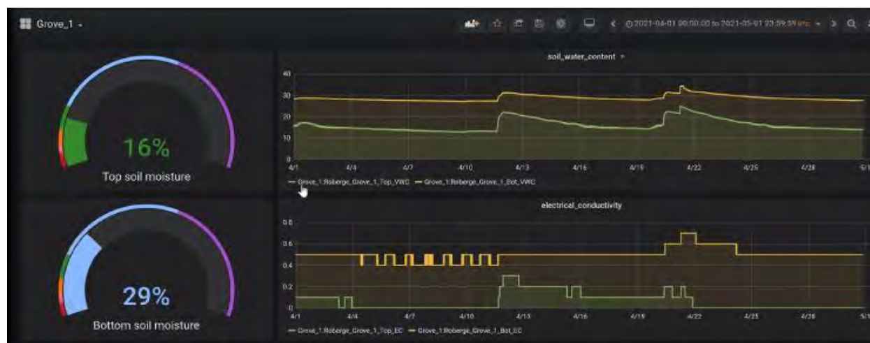
Figure 23. One of the IrrigMonitor irrigation decision support system displays. Right panel: soil moisture and soil salinity real-time data from sensors in the field. Left panel: soil moisture content based on the field soil water holding capacity conditions.
