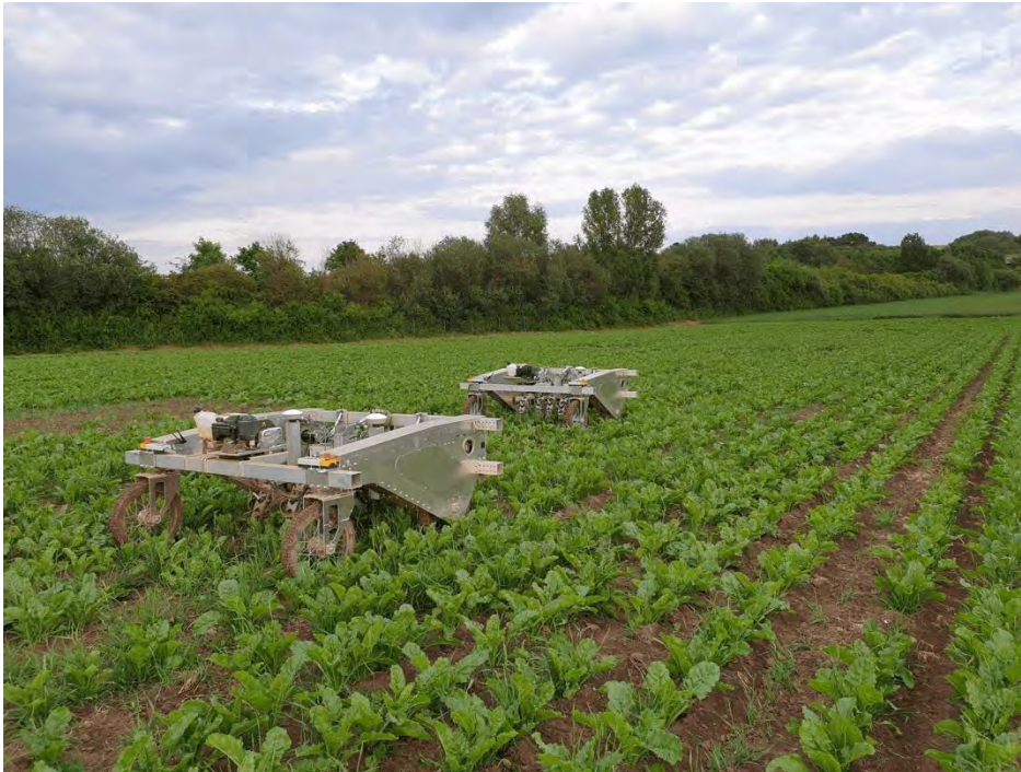
Figure 15. Autonomous robots for mechanical (non-chemical) weed control by Farming Revolution .
