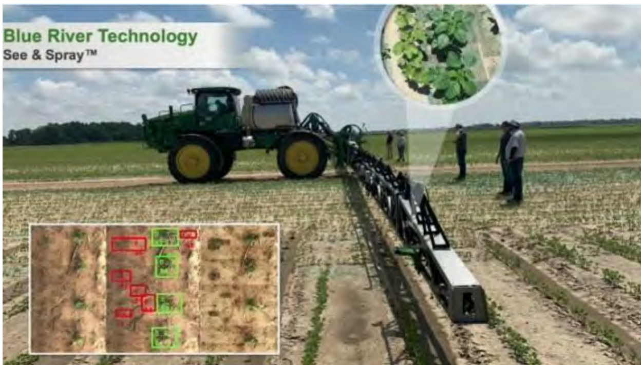
Figure 13. See & Spray technology for weed control by Blue River Technology.
