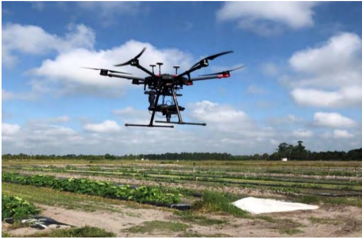
Figure 18. Unmanned aerial vehicle equipped with a hyperspectral imaging sensor.
