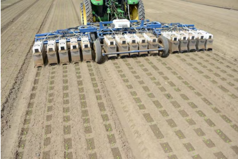
Figure 13. See & Spray technology for weed control by Blue River Technology.
