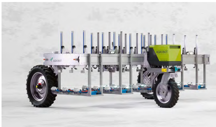
Figure 27. Agrobot harvester picks berries hanging from raised beds.
