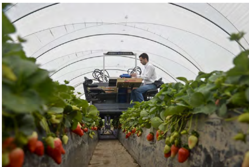
Figure 27. Agrobot harvester picks berries hanging from raised beds.
