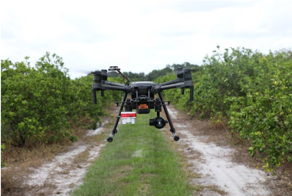
Figure 7. UAV (drone) equipped with a multispectral camera.
