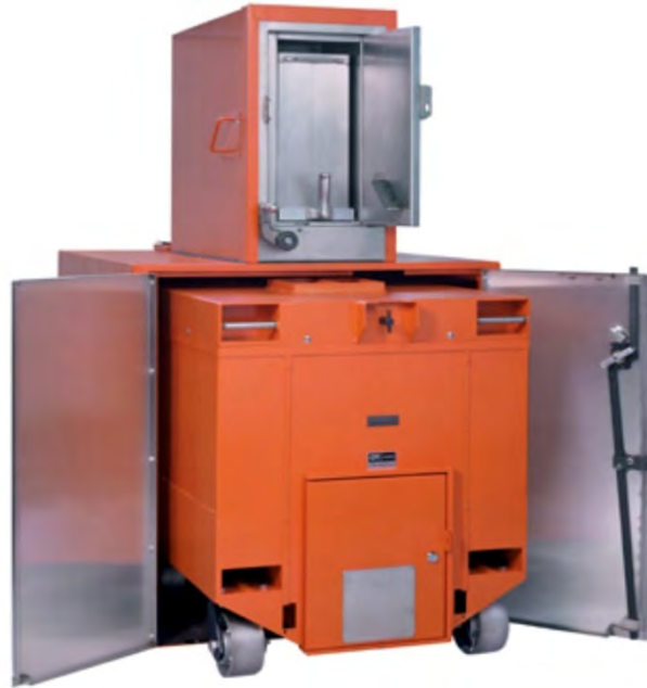
Figure 69. Mobile bin in vault housing
