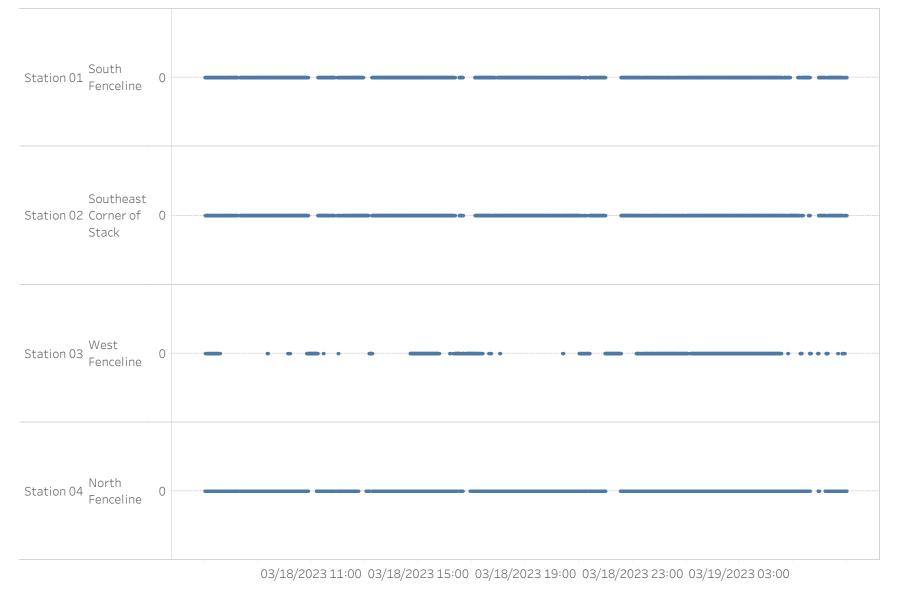
Preliminary Remote-telemetered Real-time Air Monitoring Readings PROJ-025114 | Doral Florida Facility Fire | Doral, FL 03/18/2023 07:00 to 03/19/2023 07:00 | Analyte: CO (ppm)
