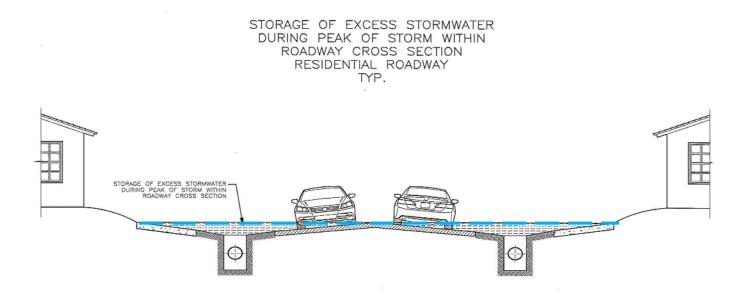
Figure 12: Roadways are designed to reduce the risk of flooding to adjacent properties by storing stormwater.
