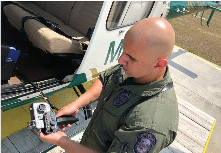
Tactical Flight Officer Teddy Alvarado demonstrates the use of the remote control unit for the high definition camera and the thermal imaging camera. (Photo by Brian Ballou)
