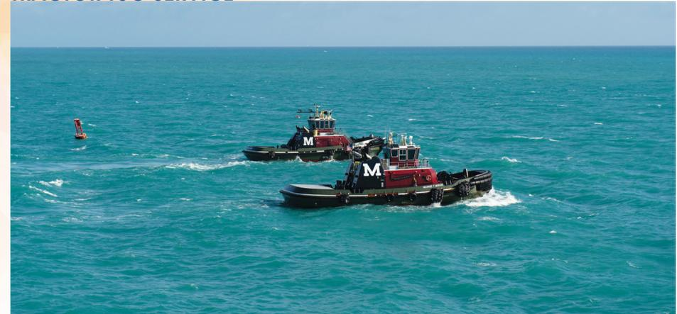
Expanded towing and harbor ship services that provide a Z – drive thrust unit with an 80 ton bollard pull and 6,700 rated horse power capacity for the berthing and departure of containerized cargo vessels.
