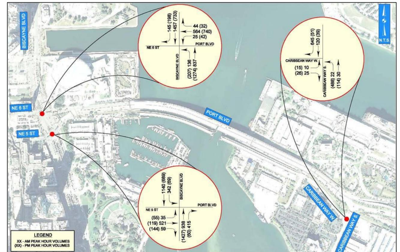
Figure 7.13 shows the existing lane configurations for the analyzed intersections.
