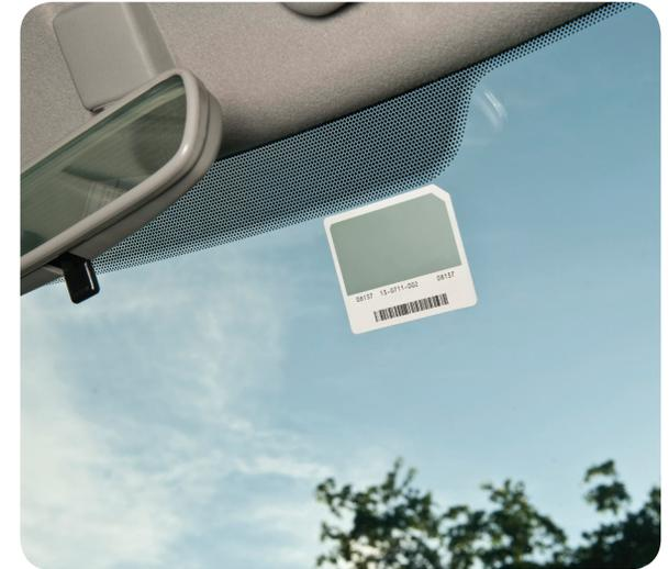
Affix the GTS Go-Pass transponder inside the windshield of your vehicle as shown. It can be placed on either side of the rear-view mirror.
