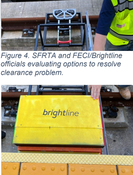
Figure 5. The rolling jig with a mock-up of the level-boarding step to be installed on Tri-Rail passenger coaches.
