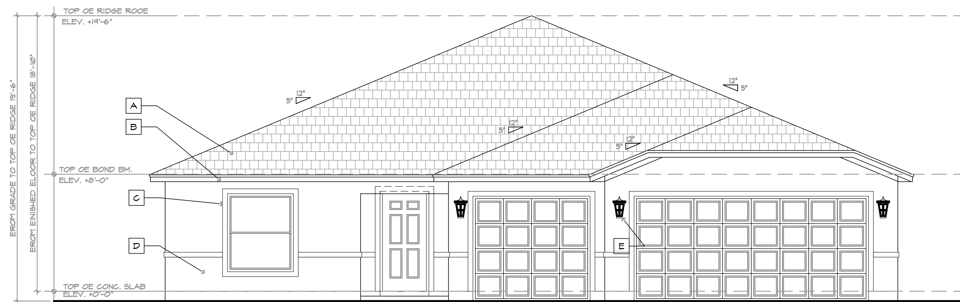
UNIT P005-HERITAGE - FRONT ELEVATION (OPTION I) SCALE: 1/4" = 1'-0"
