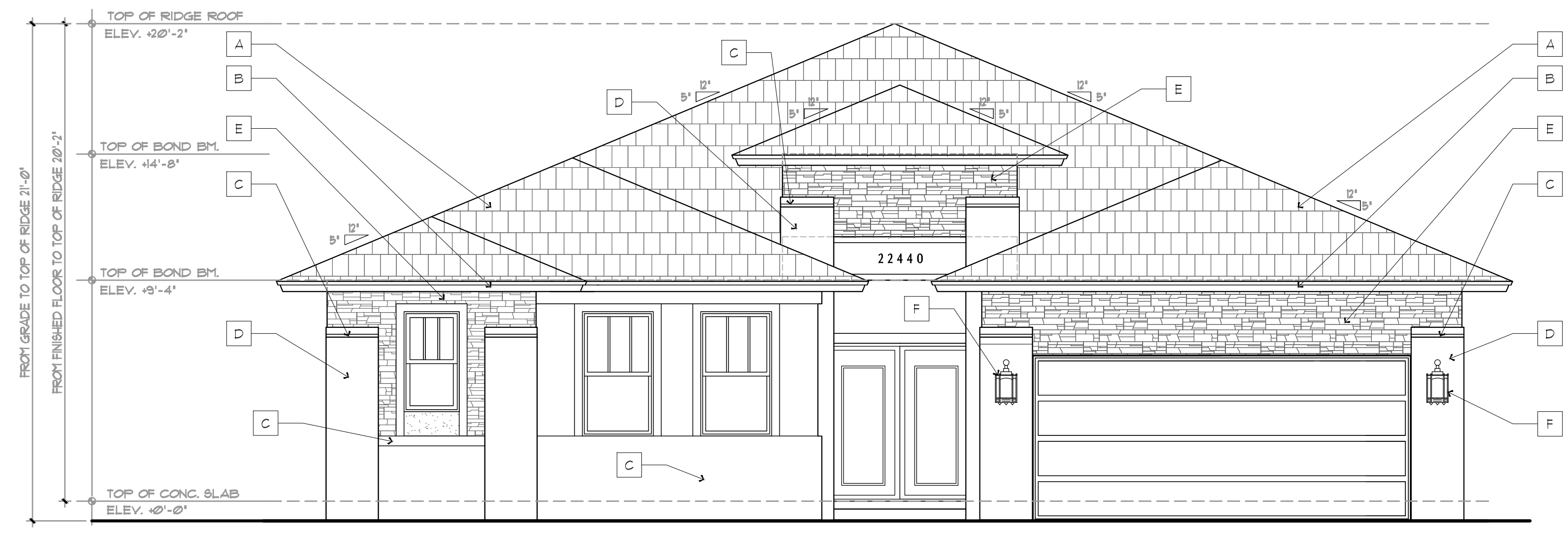
UNIT 2244 - FRONT ELEVATION SCALE: 1/4" = 1'-0"
