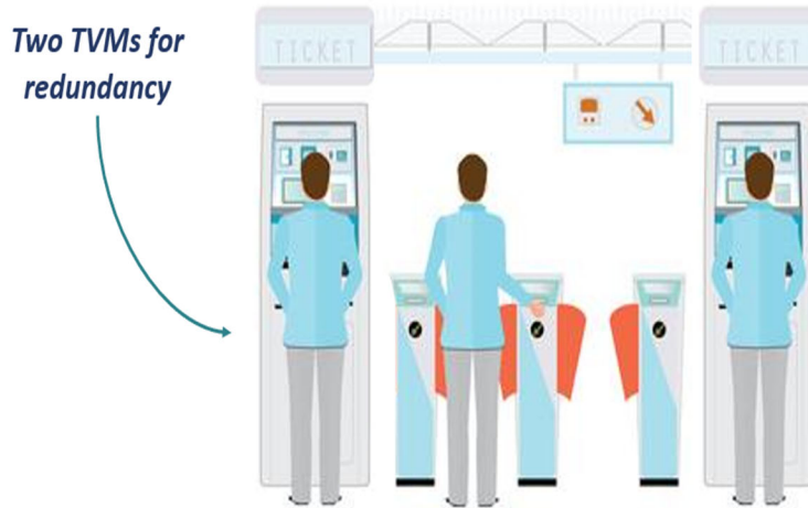
South Dade BRT Stations Two ADA Accessible Fare Gates (max 8'4" combined width) Two Slim Ticket Vending Machine (no more than 3'10" each) (Cash, Credit/Debit Card Accepted)
