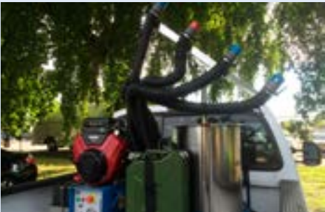
The larvicide spraying mechanism on one of the Division's new larviciding trucks.
