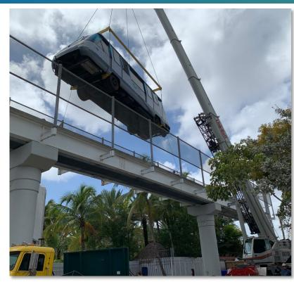
Photos showing Metromover vehicle being prepared for transport to the Alstom facility in Pittsburgh and vehicle 46 refurbishment work and testing
