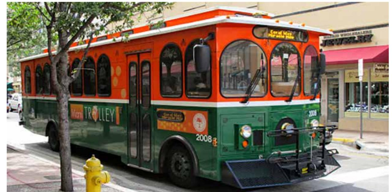
Figure 69: Most trolleys are high floor and low capacity, limiting their usefulness for high ridership service
