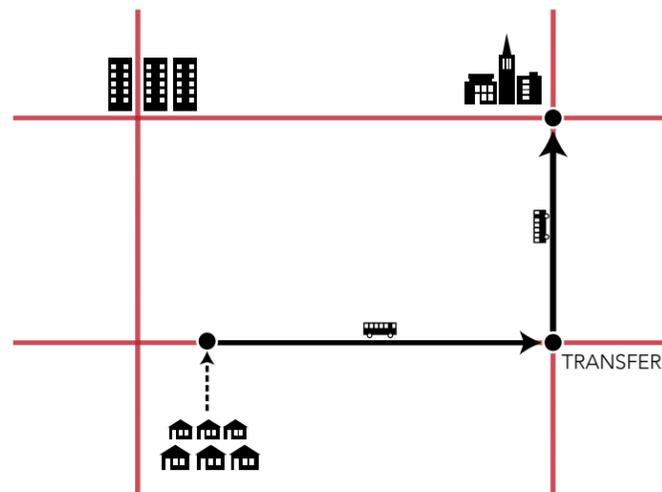
Figure 25: A grid network is a highly efficient way to connect any two destinations across a large area with a multitude origins and destinations.
