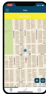
**SiBike App** sends the cyclist's location via GPS to the traffic signal. The cyclist presence has been detected.
