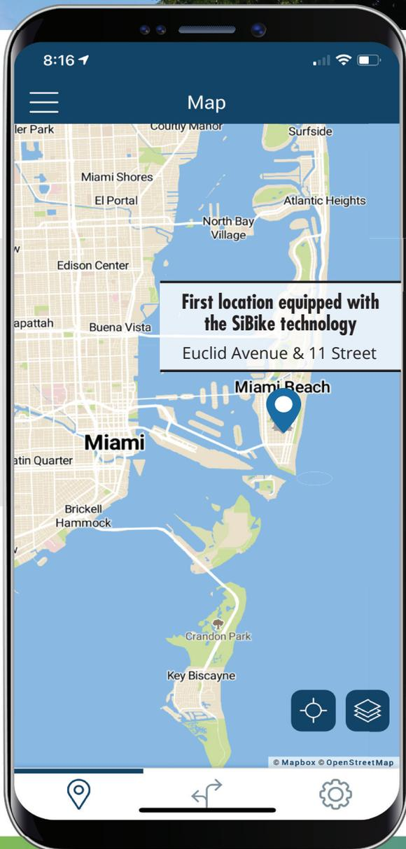
SiBike provides GPS-based bike detection through a smartphone app. Once set up, the free SiBike app knows where the bike rider is, and also what intersections have been configured to accept a bike detection message. As a result, traffic signal controllers programmed to interface with the app will detect the rider approaching the intersection and facilitate a green light for the bicyclist as soon as safely possible.
