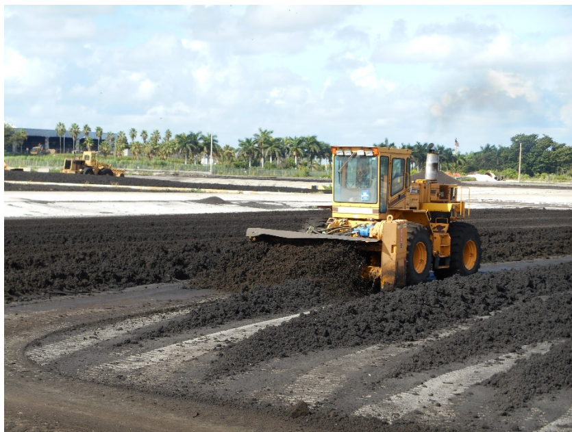
Figure 3-1. Windrow Turning at the SDWWTP Composting Facility Biosolids Market Feasibility Study
