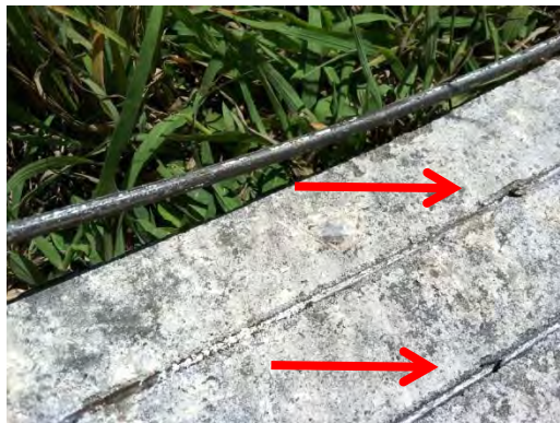
Figure 3.6 Brittle wire fractures observed embedded in a sample of the mortar coating.
